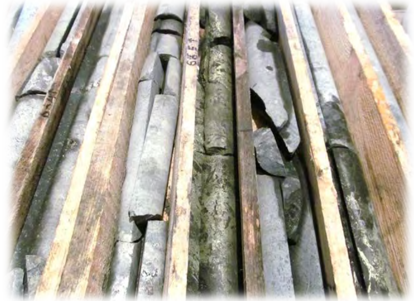
Core recovery from wells
