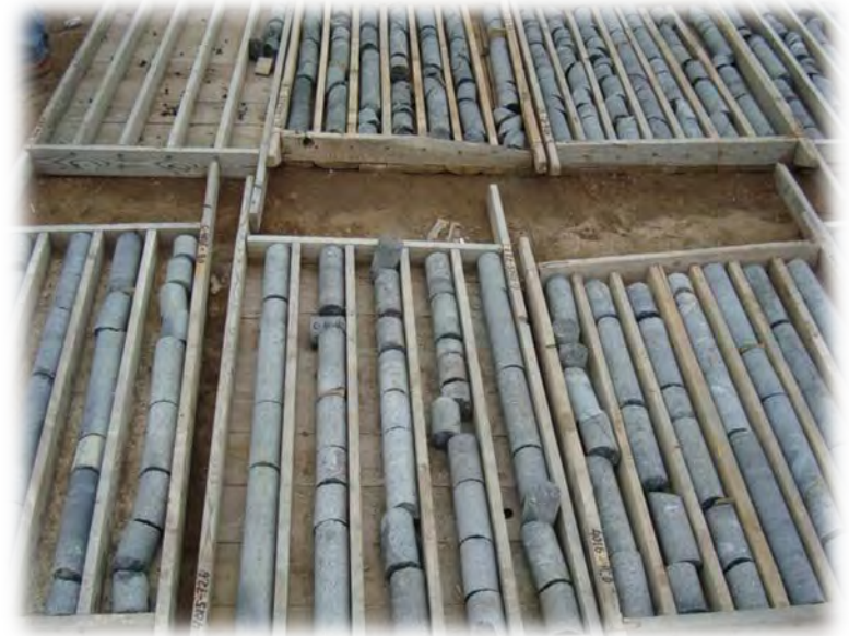
Core recovery from wells
